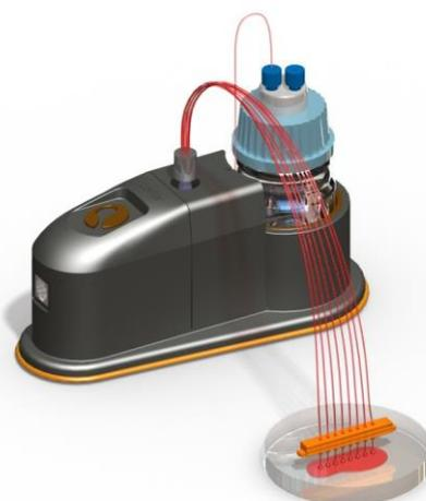
Connect tubing from media bottle to the inlet port of the pump. Connect tubing from outlet port of the pump (8 way cable with pins) to a sterile petri dish. Wash the pump using iKima App with media for 3 minutes.
